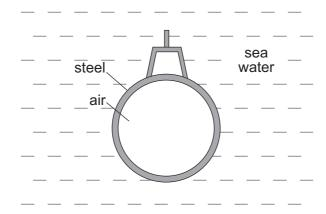
What causes the upthrust on the submarine?
