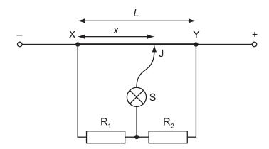
To determine the ratio  $\frac{V_1}{V_2}$  of the potential differences across R<sub>1</sub> and R<sub>2</sub>, a point is found on XY at which the lamp is off. This point is at a distance x from X.
