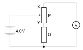
The slider on the potentiometer is moved from X to Y and a graph of voltmeter reading V is plotted against slider position.
