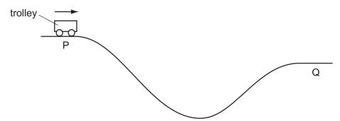
At P, the kinetic energy of the trolley is 5kJ. Between P and Q, the work the trolley does against friction is 10 kJ.
