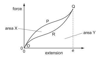
As the force is increased, the curve follows the path OPQ to extension *e*. As the force is reduced, the curve follows the path QRO to return to zero extension.
