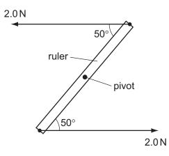
What is the magnitude of the torque of the couple on the ruler when it is in the position shown?
