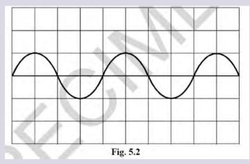
According to Faraday's law the e.m.f. included is directly proportional to the rate of change of flux linkage. In the context of this experiment, the maximum e.m.f. induced is directly proportional to the frequency of rotation of the magnet.
