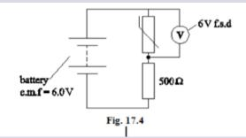
The voltmeter has very high resistance and has a full scale deflection (f.s.d.) of 6.0 V.
