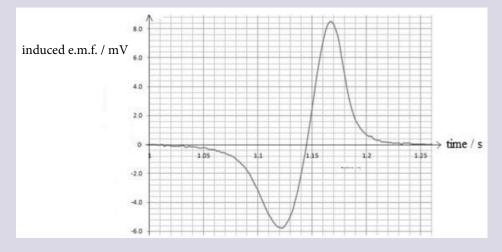
(a)\* Identify and explain the main featires of the peaks of induced emf shown on **Fig. 3.2**, in terms of Faraday's law of electromagnetic induction.
