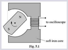
It consists of a magnet, on the shaft of a variable speed motor, being rotated inside a cavity in a soft iron core. The output from the coil, wound on the iron core, is connected to an oscilloscope. The grid of **Fig. 5.2** shows a typical output voltage which would be displayed on the oscilloscope screen.
