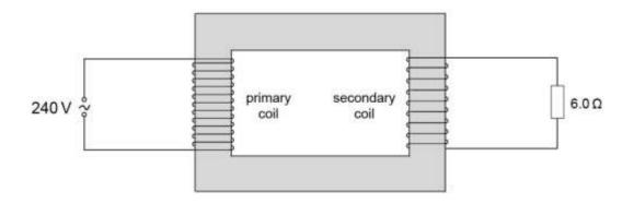
A 240V a.c. supply is connected to the primary coil and a  $6.0\Omega$  resistor is connected to the secondary coil.
