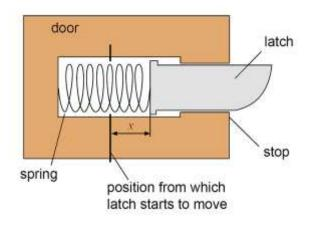
The latch is pushed in, the spring becomes compressed but remains within its elastic limit.
