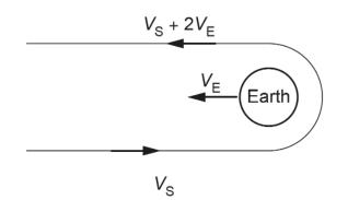
Fig. 3 Velocities of approach and recession of spacecraft to Earth, relative to the Sun.
