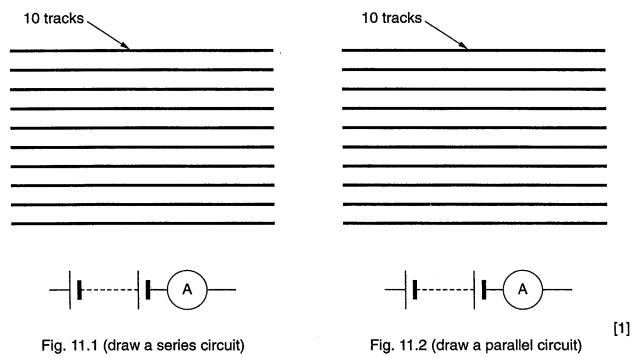
To demist effectively, each track in the heater needs to dissipate a .power of 24 W. The battery operates at 12Vd.c. (ignore the effects of internal resistance).
