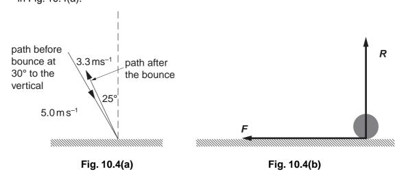
In this bounce, R is unchanged but the spinning ball experiences a greater frictional force F, as shown in Fig. 10.4(b).
