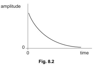
Fig. 8.2 shows how the amplitude of the standing wave decreases with time. The amplitude decreases by a factor of 0.75 every 200 vibrations of the wire.
