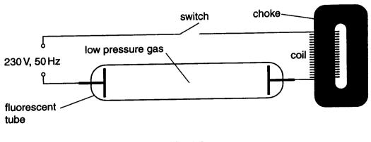
Fig. 9.2 2864/01 Jun03 The **choke** is a low resistance coil of wire wound on a loop of iron. This controls the current in the tube when it is conducting. The graph of Fig. 9.3 shows how the **flux linkage** through the choke coil changes with time when the tube is conducting.
